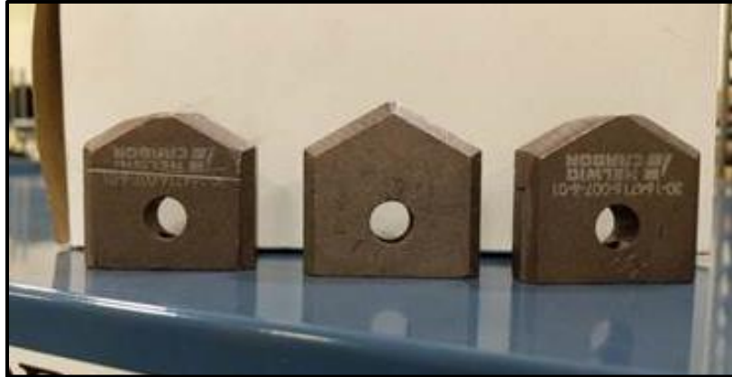
Figure 5.10: New and Used Charger Pilot Brushes (Middle) New (Left and Right) Used
