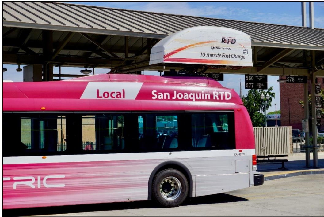
Figure 4.5: Proterra Bus Receiving On-Route Fast Charging at the Downtown Transit Center
