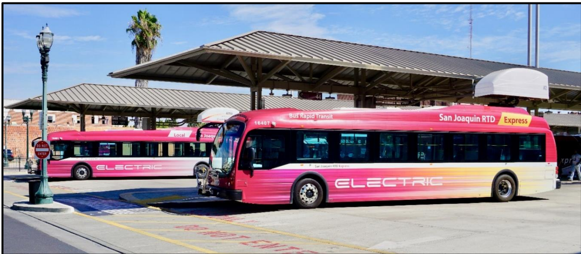
Figure 4.7: Two Buses Charging at the DTC On-Route Overhead FCrs
